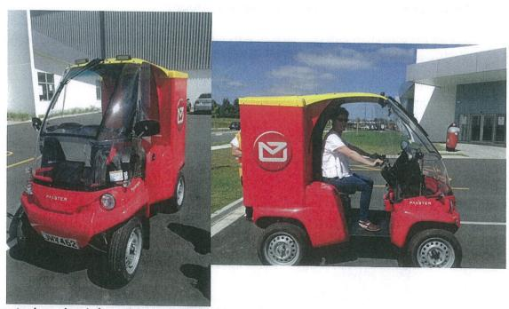
The Paxster is an electric four wheel motorbike with step through space for the driver to easily get in an out while delivering the mail.
