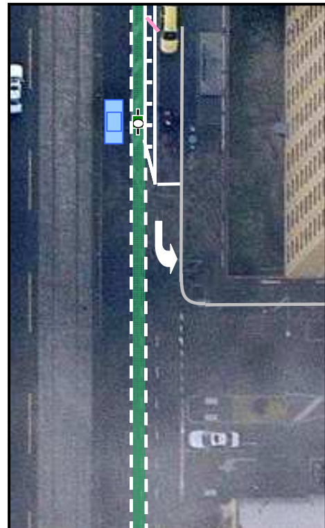
Figure 6: Intersection changes to encourage two-stage left turn: - left turn arrow - green dashed bicycle lane - bicycle lane and buffer switched
