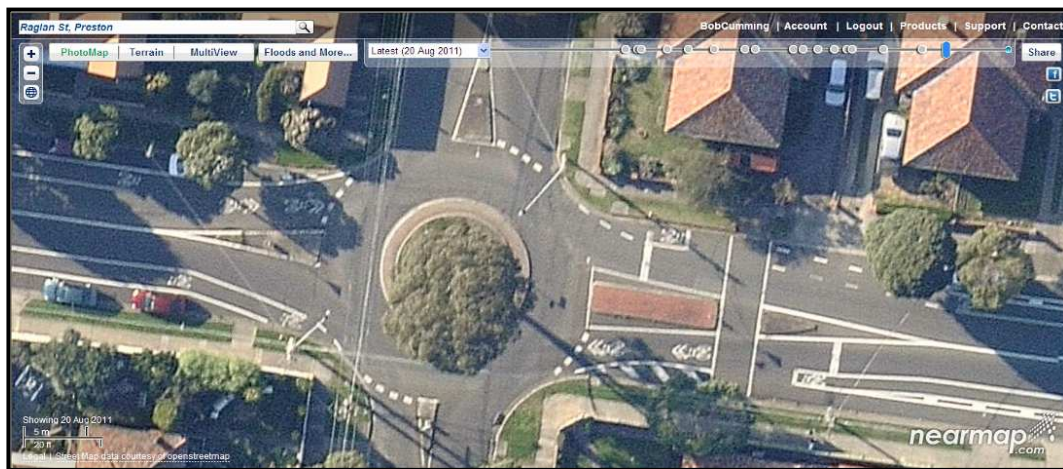
City of Darebin (Vic, Australia) – intersection of Raglan St & Hotham St, Preston. Design includes sharrows in the middle of lanes on Raglan St entries. Other examples on Raglan St. Installed July 2011.
