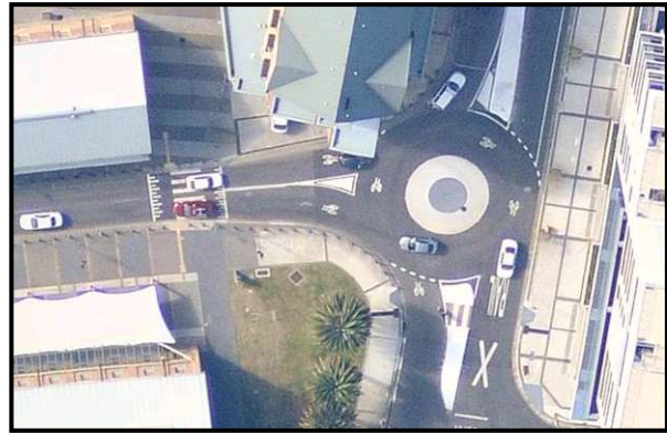
City of Newcastle (NSW, Australia) Prince St & Platt St, Waratah Honeysuckle Dr & Merewether St, Newcastle. Designs includes bicycle logos in middle of lanes (entry and circulating). Installed May 2011
