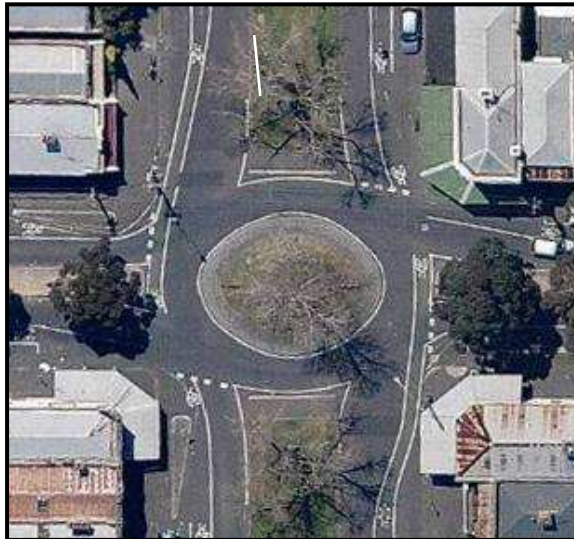
2009: roundabout with circulating bicycle lanes.
