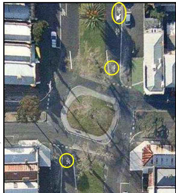
2012: Changed roundabout with features to encourage cyclists to merge with cars and use primary position: - 45° bicycle lane arrow to encourage merging to the centre - Centrally positioned bike logos at entries - circled - Kerb extensions to force greater deflection by cyclists
