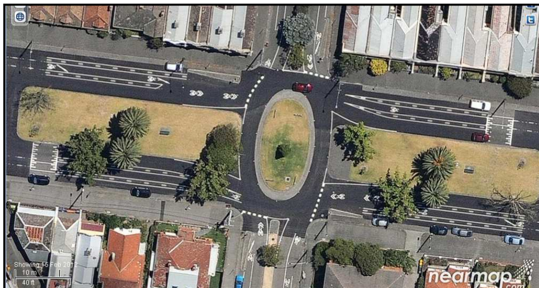
City of Yarra (Vic, Australia) – intersection of Pigdon St & Garton St, Carlton. Design includes: sharrows in middle of lanes on all entries; bicycle symbols with merge arrows on all approaches; safety strips between parking, bicycle lanes and car lanes on Pigdon Street; and narrow driving lanes – for lower speeds. Other examples exist on Pigdon St. Installed Feb 2012.
