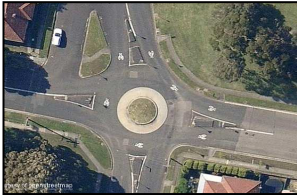
City of Newcastle (NSW, Australia) Prince St & Platt St, Waratah Honeysuckle Dr & Merewether St, Newcastle. Designs includes bicycle logos in middle of lanes (entry and circulating). Installed May 2011
