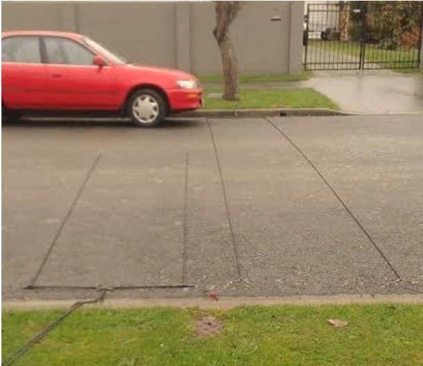
Figure 4. Road tubes configuration on Hinau Street
