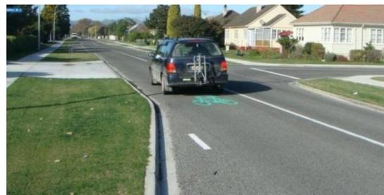
Figure 31: Green cycle symbol in centre of narrow lane at pinch point, Hastings
