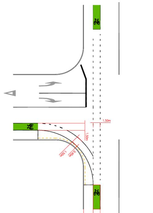
Figure 44: Coloured is used before and after side road junctions, Palmerston North
