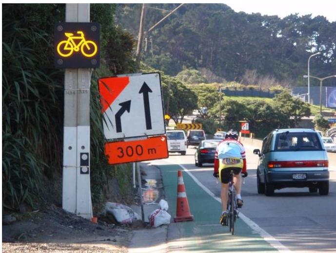
Figure 58: Example of an active sign
