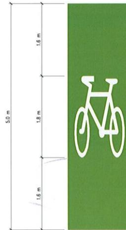
Figure 39: Proposed Auckland Transport cycle lane marking
