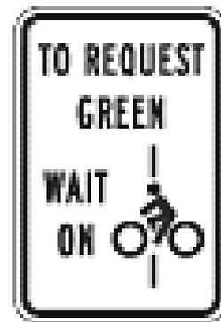
**Figure 47: MUTCD Figure 9B-2 Regulatory Bicycle Facility Sign R10-22 (optional)**
