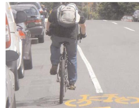
Figure 15: A BAZ marking (with lane line and parallel parking)
