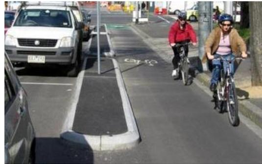
Figure 12: Kerb protected cycle lane, Melbourne
