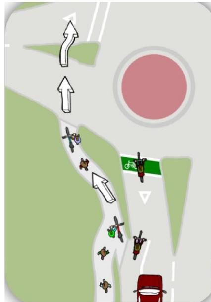
Figure 25: Cycle friendly roundabout proposal (Hastings)
