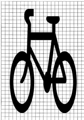
**Figure 4: M2-3 cycle symbol as defined in the TCD Rule**
