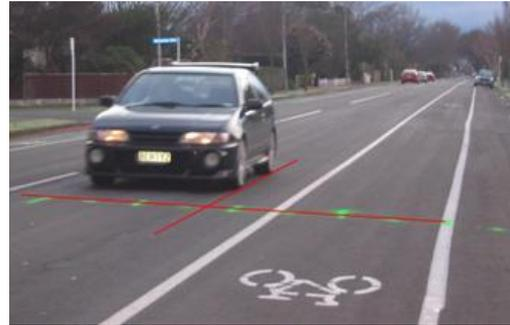
Figure 43: Research on lane positioning with and without green cycle lane colour, Palmerston North
