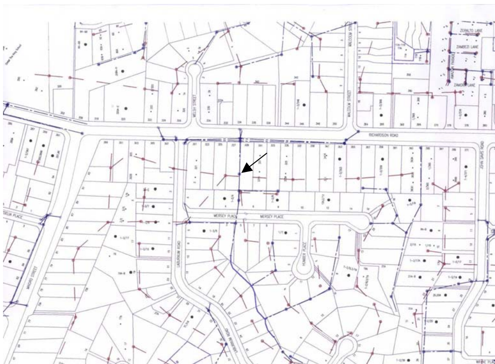
Figure 7. Stormwater network at Richardson Road. Arrow shows monitoring point.
