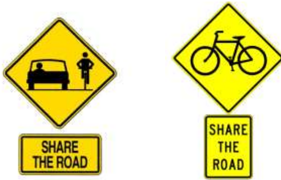
Figure 3: Example of a “Share the Road” signs
